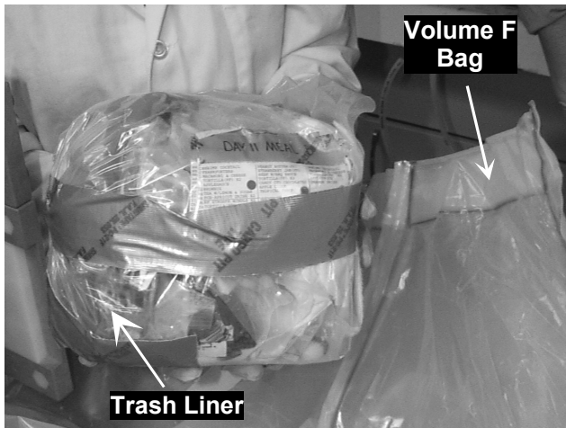
Figure 1. Volume F Bag Access Opening and Trash Liner Filled With Plastic and Plate Wastes
